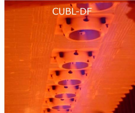
Typical Furnace Operating Temperature 1800 to 1900 Deg. F.
