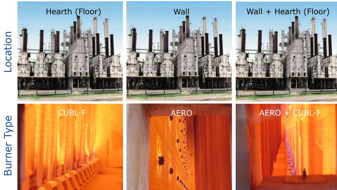
Typical Furnace Operating Temperature 2200 to 2300 Deg. F.
