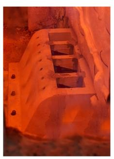
CUBP Steam Cracker Burner Firing 100% Hydrogen
